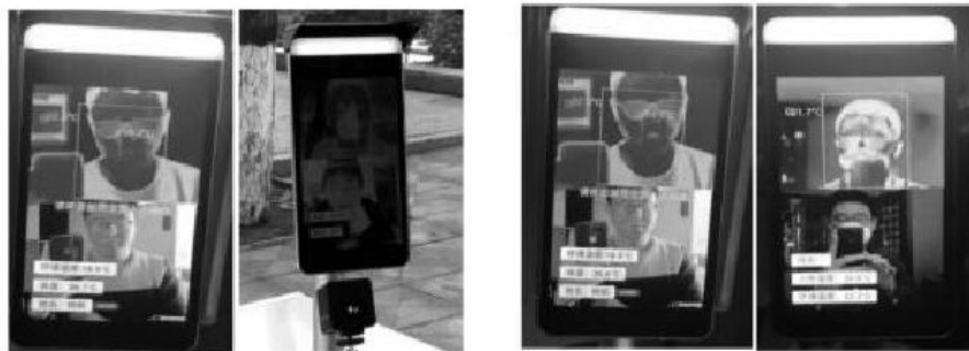
Figure 1. Face recognition and body temperature detection in the student dormitory gate system [4]
