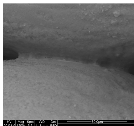
Fig. 2 Unmodified bonding bridge
