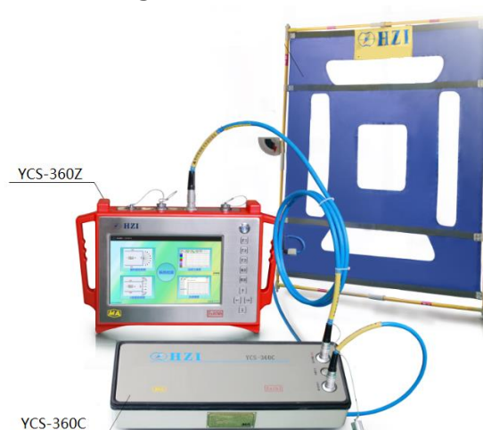
Fig.1 YCS360 mine multi-channel transient electromagnetic instrument system
