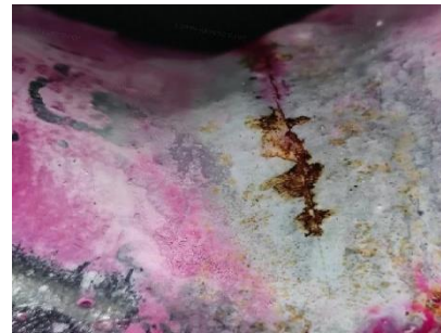
Figure 16: Subframe stress concentration area (enhanced road test site durability test)
