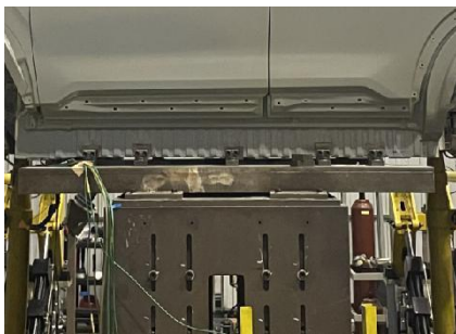
Figure 7: Fixing method of side beam
