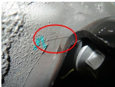
Figure 15: Subframe stress concentration area (road simulation durability test)
