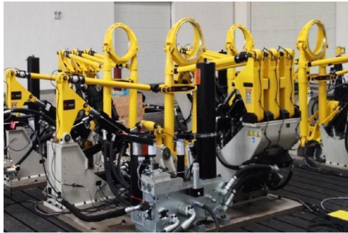
Figure 1: 6-DOF spindle-coupled road simulation test bench
