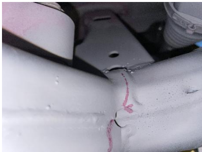
Figure 15: Subframe stress concentration area (road simulation durability test)
