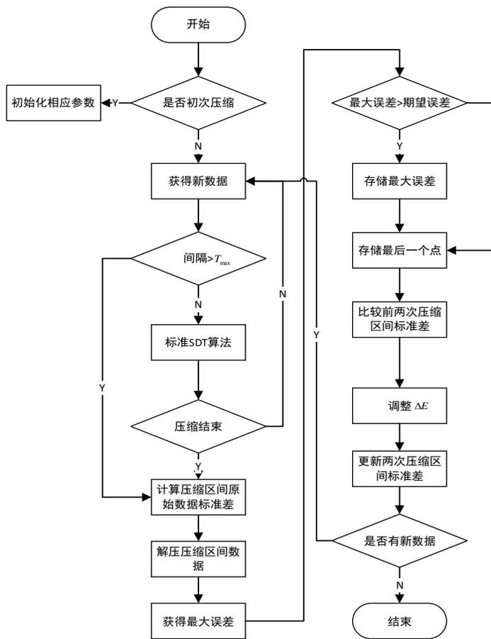
Figure 2 Improved algorithm flow
