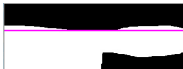
Figure 8: Oil level line of conservator
