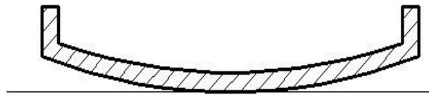
Figure 2 Positive deformation of single-sided frame parts after processing
