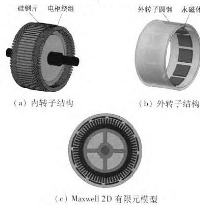
Figure 3. Schematic diagram of stator and rotor structure
