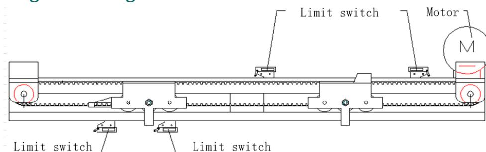
Fig. 1 Control system with limit switch
