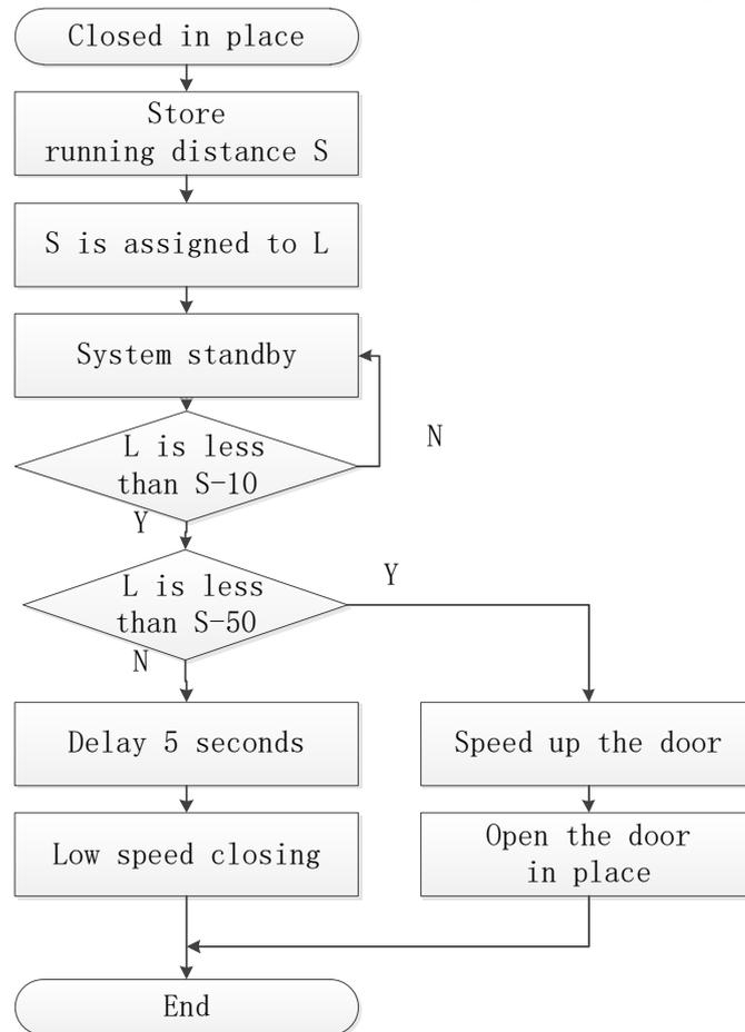
Fig. 3 Complete process of self-locking function
