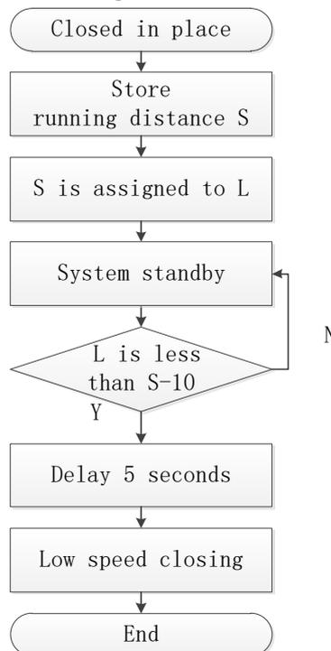
Fig. 2 Self-locking function
