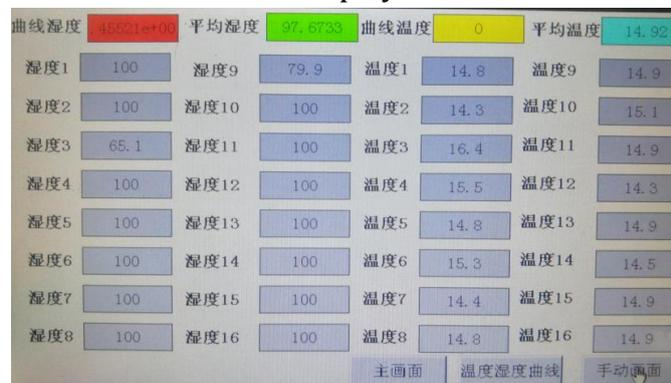
Figure 2-3 Daqu fermentation room temperature and humidity current value display interface
