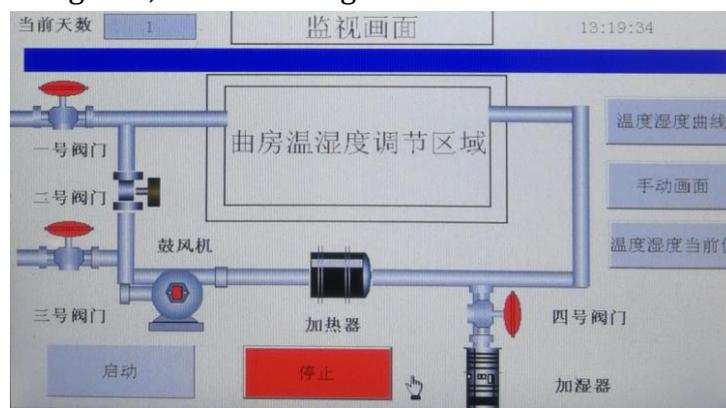
Figure 1-7 Automatic control interface of skid-mounted Daqu fermentation room
