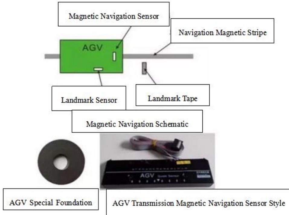
Figure 1: Magnetic navigation system diagram
