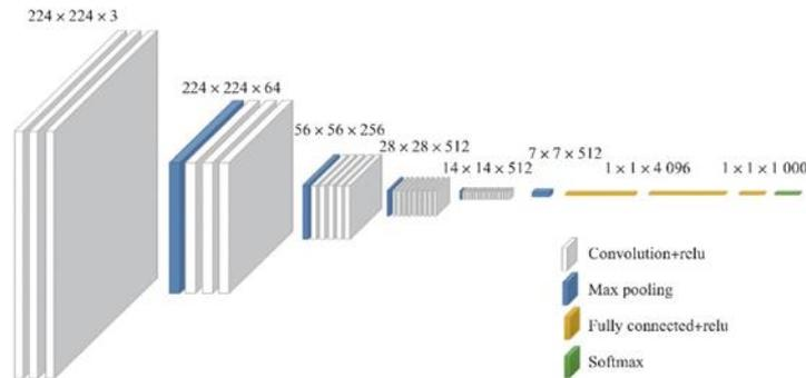
Figure 1: VGG16 network structure
