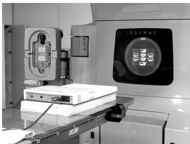
Figure 5 MatriXX two-dimensional ionization chamber dot matrix
