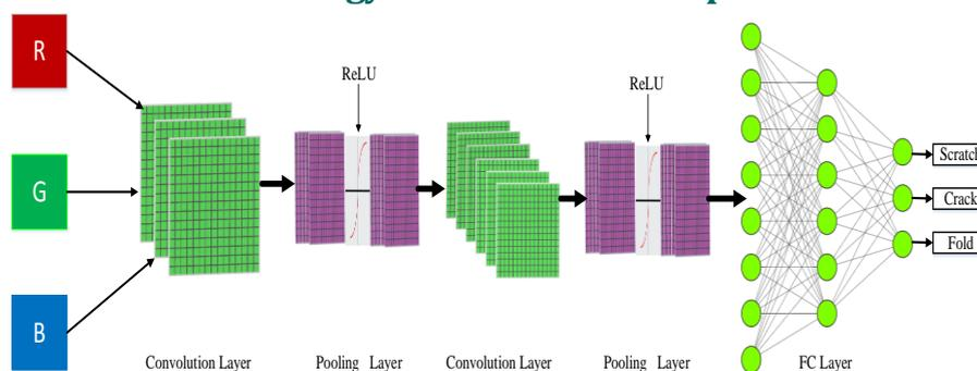
Figure 1 Defect detection model based on CNNs
