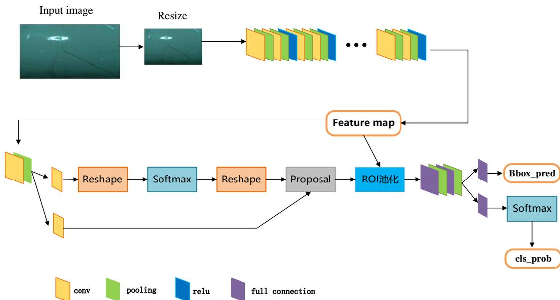
Figure 2 Fast R-CNN model structure
